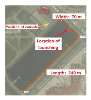
Figure 9. The test environment.
