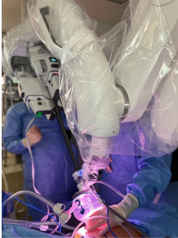
**Figure 1.** An overview of the Da Vinci SP® surgical system: a single instrument arm, including four instrument drives in which to insert the endoscope and three double-jointed articulating robotic instruments. SP: Single port.
