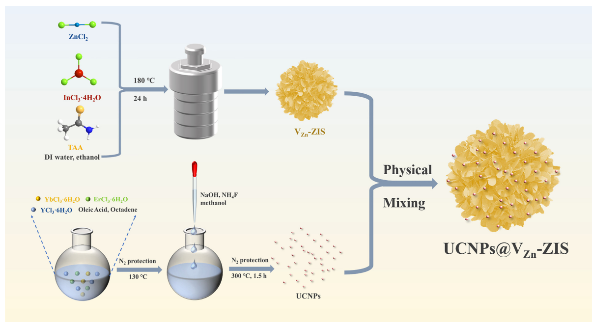
Figure 1. The synthesis procedure of composite of UCNPs@V Zn -ZIS. UCNPs: Up-conversion nanoparticles; V Zn -ZIS: Zn vacancy-rich ZnIn 2 S 4 .
