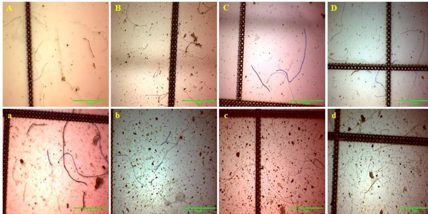
**Figure 2.** Microscopic images of isolated microfibers from different treatment groups of freshwater [(A) 400 ml FW; (B) 40 mL 95% alcohol + 800 mL FW; (C) 40 mL 30% H<sub>2</sub>O<sub>2</sub> + 800 mL FW; and (D) 4 g SDS + 800 mL FW] and saltwater [(a) 800 mL SW; (b) 40 mL 95% alcohol + 800 mL SW; (c) 40 mL 30% H<sub>2</sub>O<sub>2</sub> + 800 mL SW; and (d) 4 g SDS + 800 mL SW]. Scale bar: 1 mm; and zoom: 4X.
