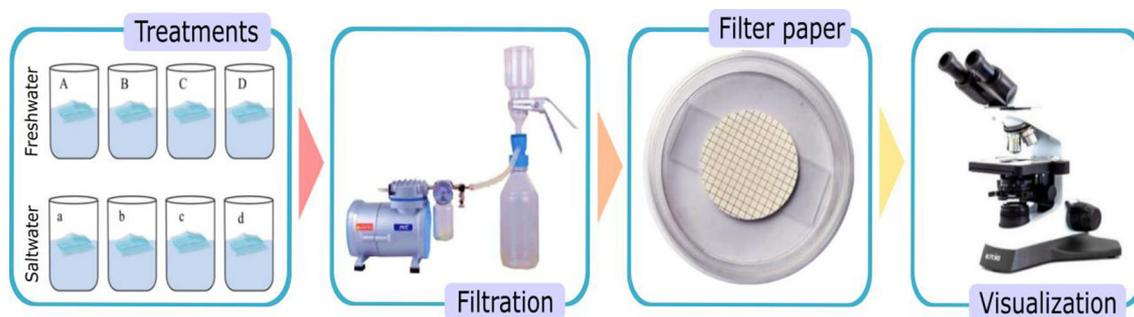
**Figure 1.** The treatments, filtration and visualization process for microfiber extraction.
