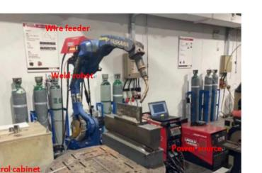
Figure 13. Robot system.
