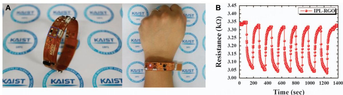
Figure 21. (A) Photograph of wearable sensor (the flexible IPL-RGO sensor layer is in the blue box); (B) the sensor has stable H 2 S sensing performance [17] .
