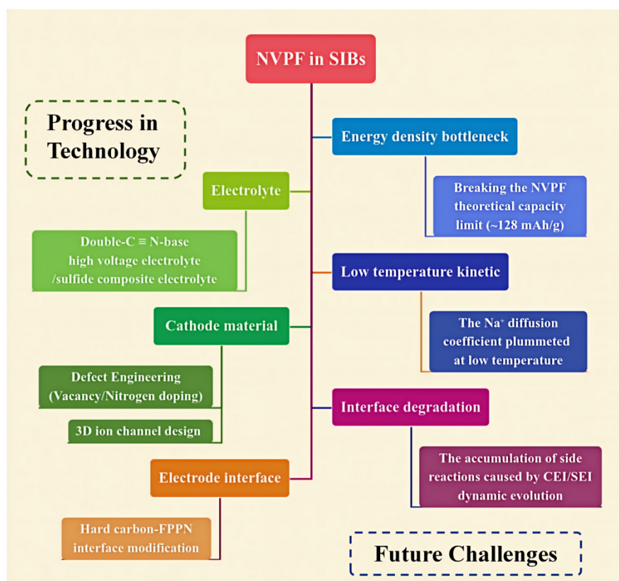
Figure 9. The progress in technology and future challenges of NVPF in SIBs. NVPF: \text{Na}_3\text{V}_2(\text{PO}_4)_2\text{F}_3 ; SIB: sodium-ion battery; SEI: solid electrolyte interphase; CEI: cathode-electrolyte interface.
