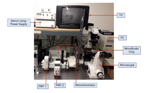
Figure 2. Nikon-PTI optical measurement-imaging system setup. PMT: photomultiplier tube
