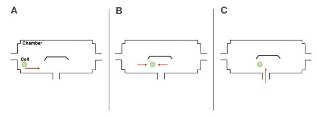
**Figure 3.** Schematic diagrams displaying how a single breast cancer cell was sorted and retained near the cell retention structure. A: Cell suspension was inserted through Reservoir 1; B: The liquid level of Reservoirs 1 and 3 was adjusted to make the cell stop near the cell retention structure; C: Upon cell retention, chemical reagents were administrated through Reservoir 2
