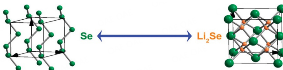
Figure 2. Structural representations of trigonal Se and antifluorite \text{Li}_2\text{Se} [11] . Copyright 2012, American Chemical Society.
