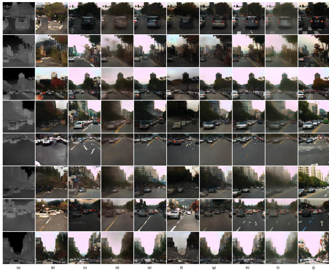
Figure 5. Colorized images using different image colorization methods on KAIST. (A) TIR images; (B) CycleGAN [33]; (C) Pix2pix [23]; (D) SCGAN [29]; (E) TIC-CGAN [28]; (F) PealGAN [32]; (G) MUGAN [30]; (H) LKAT-GAN [31]; (I) CMMF-Net; (J) True RGB images. The original infrared images (A) and RGB images (J) were obtained from https://soonminhwang.github.io/rgbt-ped-detection/data/ , while the other images were reproduced using methods from other papers and generated with our laboratory's equipment. The specific methods can be found in the corresponding references listed in the bibliography. KAIST: A multispectral pedestrian dataset, proposed by the Korea Advanced Institute of Science and Technology; TIR: thermal infrared; SCGAN: saliency map-guided colorization with generative adversarial network; TIC-CGAN: thermal infrared colorization via conditional generative adversarial network; MUGAN: thermal infrared image colorization using xixed-skipping UNet and generative adversarial network; LKAT-GAN: a GAN for thermal infrared image colorization based on large kernel and attentionUNet-transformer; CMMF-Net: a generative network based on clip-guided multi-modal feature fusion for thermal infrared image colorization.
