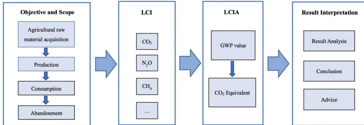
**Figure 1.** Procedure of carbon footprint measuring based on LCA. Notes: 1. LCI includes life cycle material input and corresponding greenhouse gas output. 2. LCIA converts gases with different greenhouse effects into emissions equivalent to the greenhouse effect of CO<sub>2</sub>.
