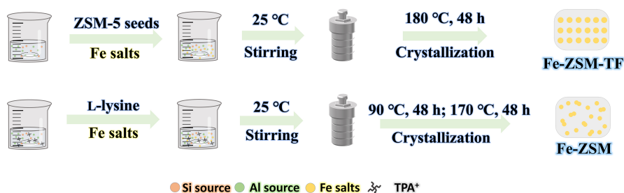
Figure 2. Schematic illustration of post-treatment and in situ synthesis methods of Fe-containing zeolite catalysts. Compared to IE, SSIE, and in situ synthesis methods, the WI method tends to cause metal particle agglomeration. IE: Ion-exchange; SSIE: solid-state ion-exchange; WI: wet impregnation.
