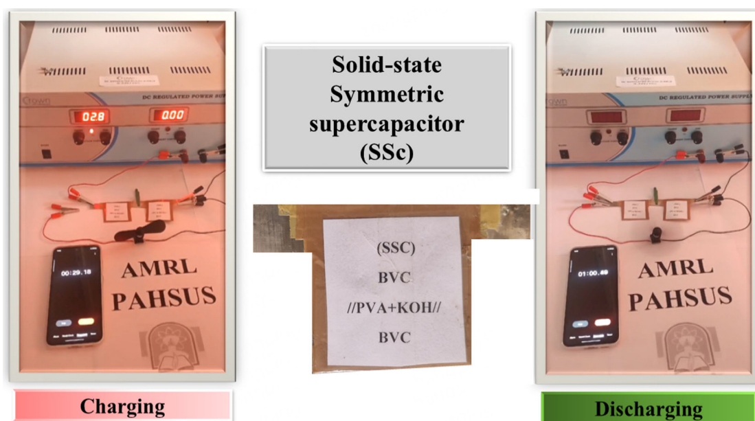
Figure 11. Photographs of the practical application of rotating the fan using the SSc device of BVC in charging and discharging mode. BVC: Bismuth vanadate/carbon; SSc: solid-state symmetric supercapacitor.
