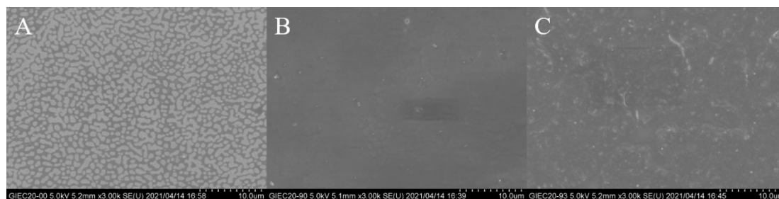
Figure 9. SEM images of PT (A), PTT (B) and PDTT (C) polymerized electrochemically on ITO-coated glass. SEM: Scanning electron microscopy; PT: polythiophene; PTT: poly(thieno[3,2-b]thiophene); PDTT: poly(dithieno[3,2-b:2',3'-d]thiophene); ITO: indium tin oxide.
