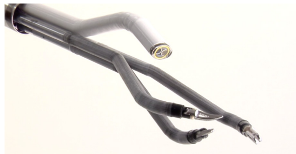
Figure 5. Angulation of single port robotic instruments employed through the single port trocar
