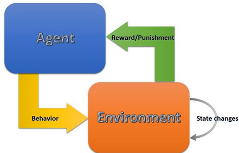
Figure 9. Universal model of RL. RL: Reinforcement learning.
