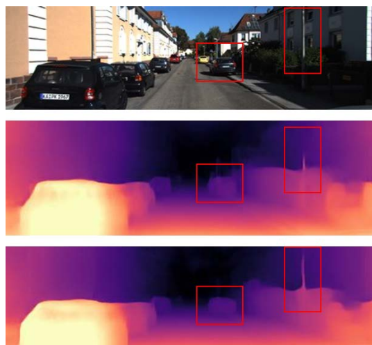
Figure 1. The input image from the KITTI dataset (top); the baseline MonoDepth2 [22] (M, ResNet50, without pre-training) depth prediction; (middle) and our result (bottom).
