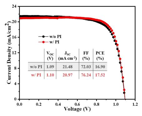
**Supplementary Figure 6.** *J-V* curve of flexible PSCs with or without PI based on polyethylene naphthalate (PEN)/ITO substrate.
