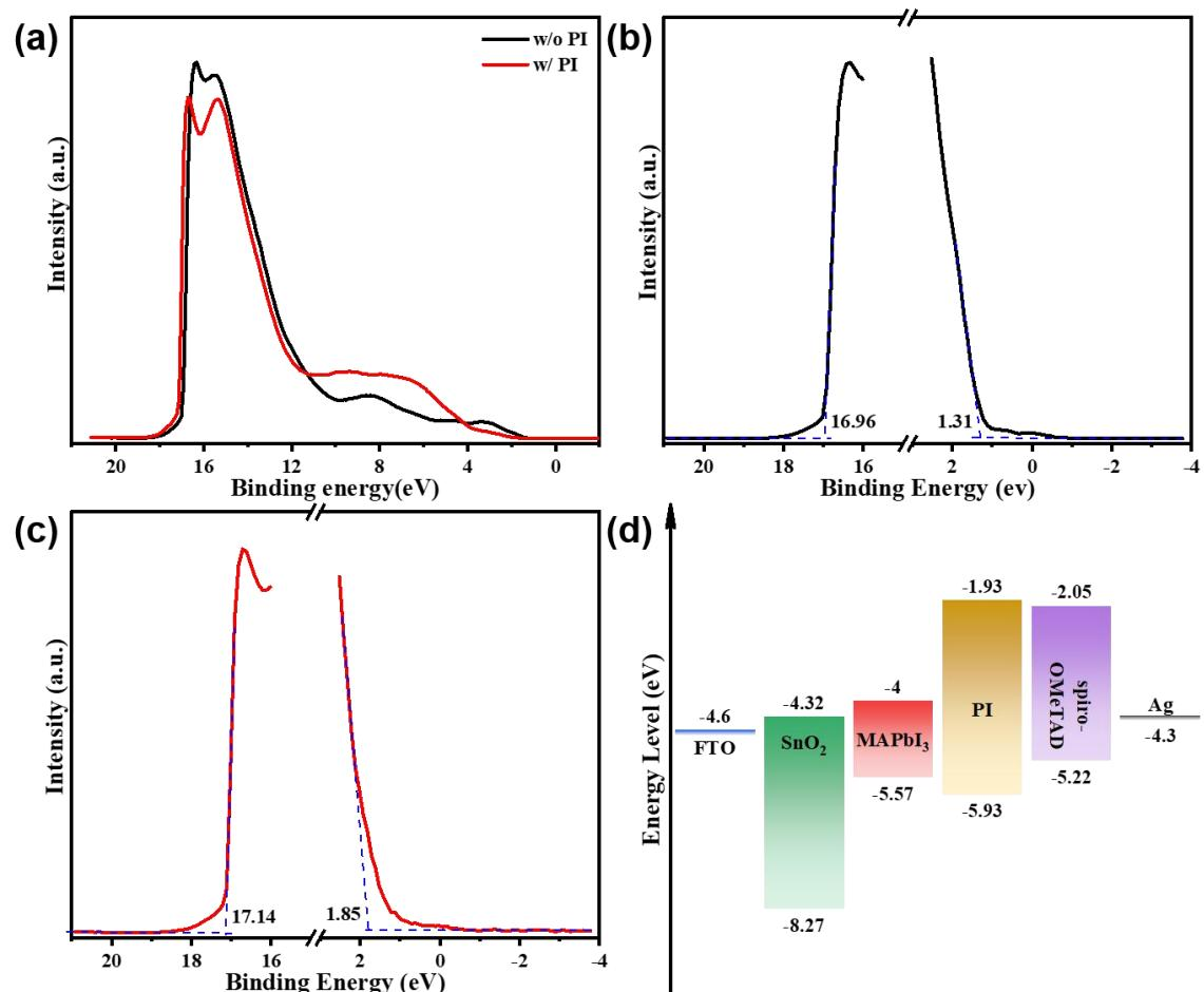
23 **Supplementary Figure 2.** (A) UPS spectrum of perovskite film without and with PI
