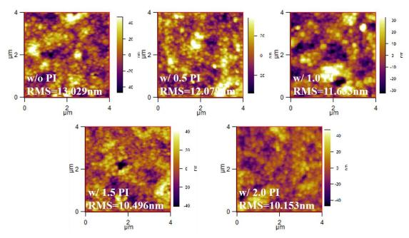
Supplementary Figure 1. AFM photos of perovskite films with different concentration
