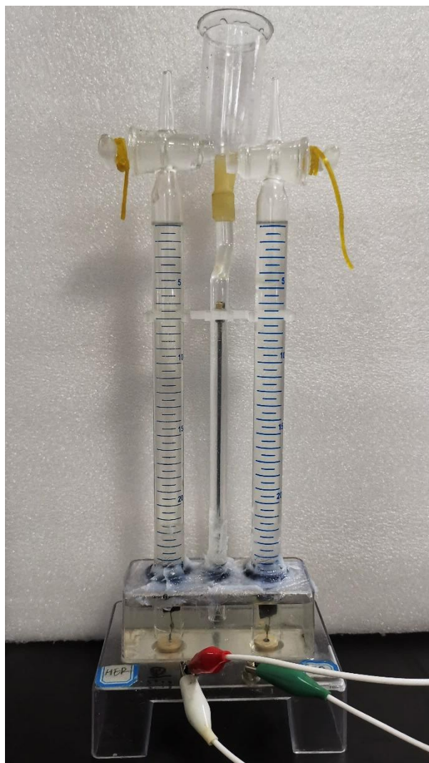
Supplementary Figure 22. The gas collecting device of evolved \text{H}_2 and \text{O}_2 .
